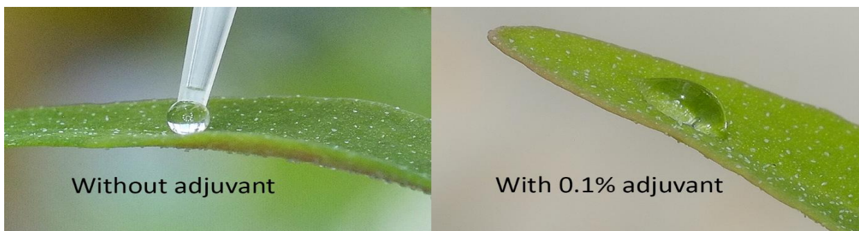
Figure 2. Droplet of 1 \mu\text{l} of deionized water applied on the waxy surface of a Chenopodium album leaf without an adjuvant (left) and with 0.1% AS 500 SL adjuvant (left).
